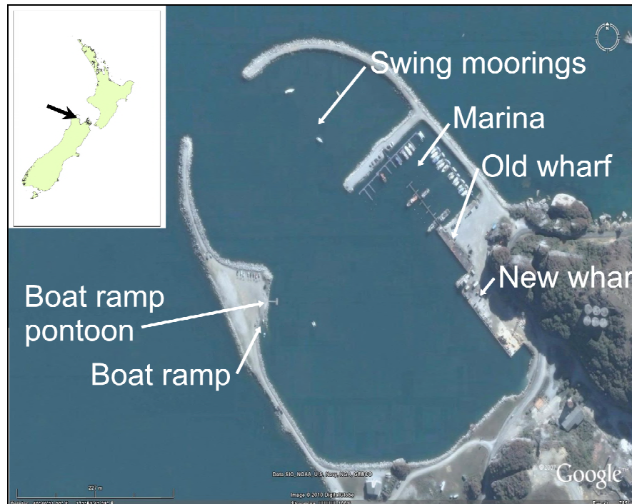
Figure 1: The location of Port Tarakohe at the top of the South Island, New Zealand, and features of the port. Note that a 70-m long extension to the western breakwall is not shown in this image. This extension is located to the north of the boat ramp area, runs perpendicular to the main breakwall, and mirrors the extension on the eastern side that protects the north side of the marina.
